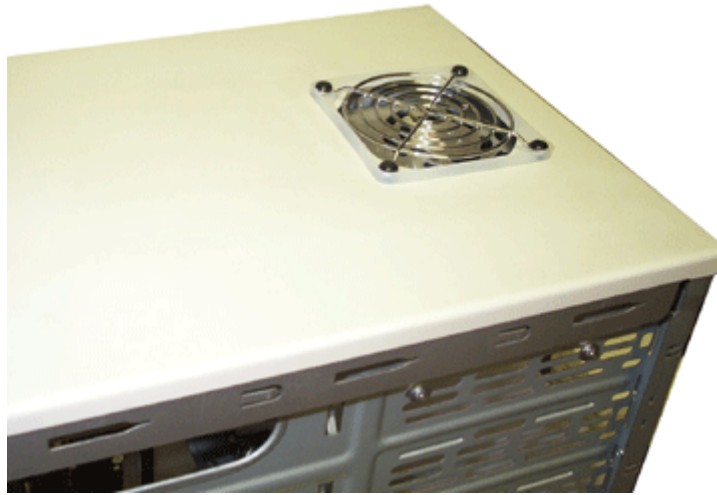
Another example of “blow-hole” installation
